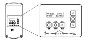
The RDC2 controller provides integrated control for the generator set, Kohler® Model RXT transfer switch, programmable interface module (PIM), and load management.
